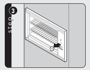
Remove all knobs, push buttons, and bezels on the right control panel.
